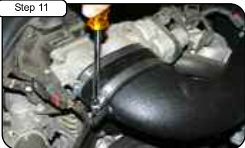
Tighten clamps with 5/16" nut driver.
