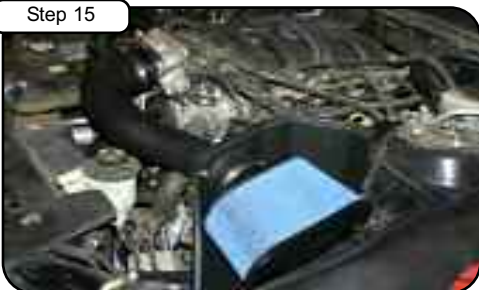
Your installation is now complete. Please check all bolts and clamps periodically. Re-tighten if necessary. Thank you for choosing aFe! Place enclosed CARB EO sticker on a clean/smooth surface on or near the device. EO identification label is required in passing the smog check inspection.
