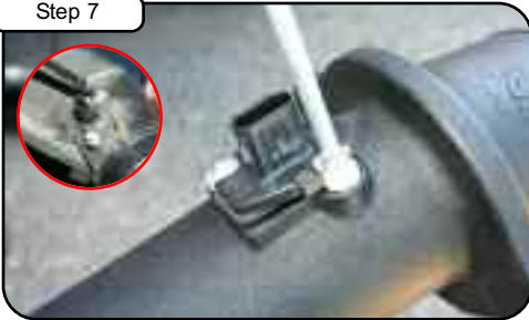
With T-20 torx bit remove MAF sensor and (with gasket, nylon spacers and screws provided) install into new tube. Make sure gasket and nylon spacers are between sensor and tube.
