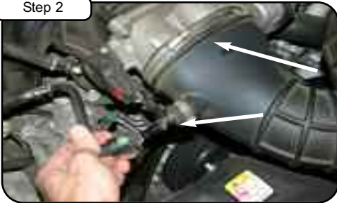
With 5/16" nut driver loosen clamp at throttle body. Disconnect and remove OE crank case line.
