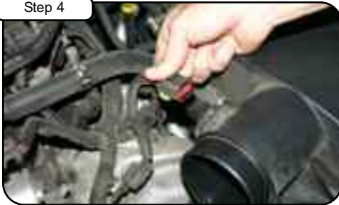
Disconnect MAF sensor harness.
