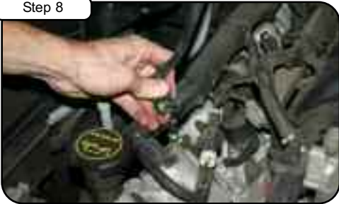
Remove factory crank case line from engine.
